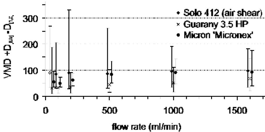
Fig. 3. Motorised mistblowers: machinery factors. The  $VMD + D_{[9,0]} - D_{[1,0]}$  is shown using water + 1% 'Codacide' from three motorised mistblowers at flow rates of 50, 100, 200, 500, 1000 and 1600 ml/min.
