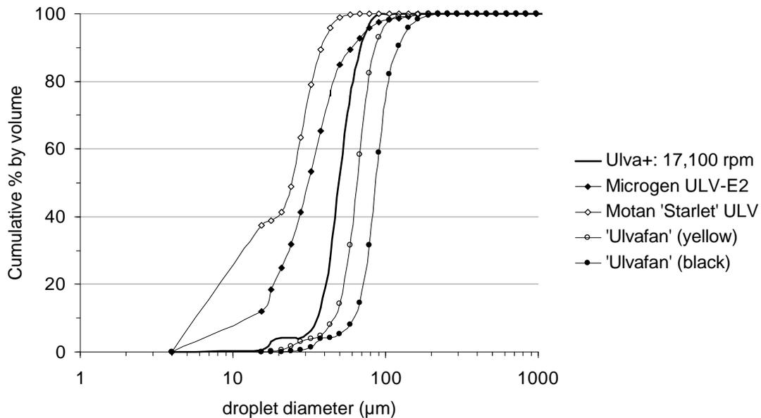
Fig. 3 Droplet spectra of two 'cold foggers' and the 'Ulvafan'
