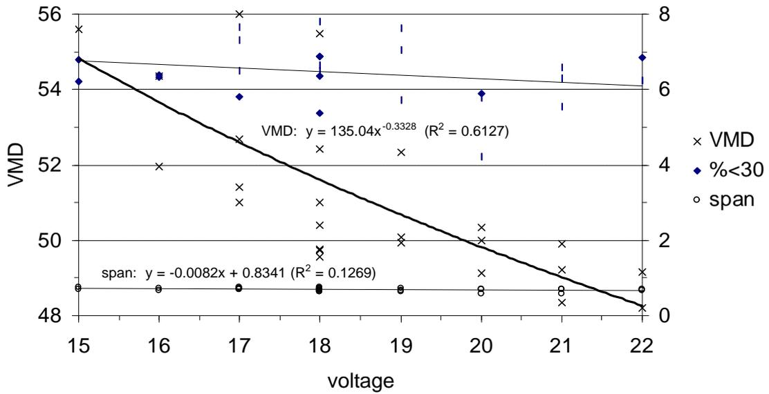
Fig. 1 Regressions for VMD and relative span for an Ulva+ loaded at 35 ml/min (yellow restrictor)
