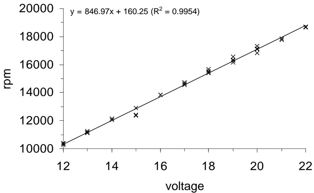
Fig. 2 Measured rotational speeds of an Ulva+ loaded at 35 ml/min (yellow restrictor)
