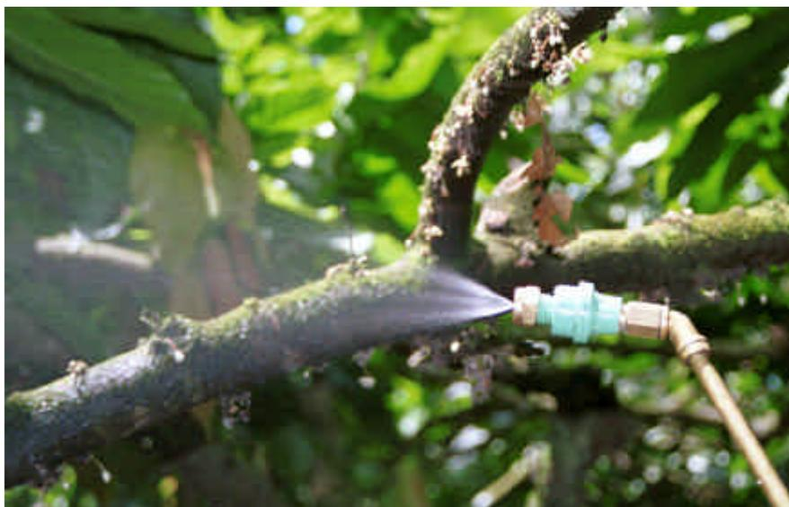
A cocoa pod nozzle in use during field trials in Costa Rica. Optimisation of nozzles to produce a very narrow angle (25-35°) and low flow rates substantially improved deposits on pods (per volume emitted) and should reduce pesticide costs.
