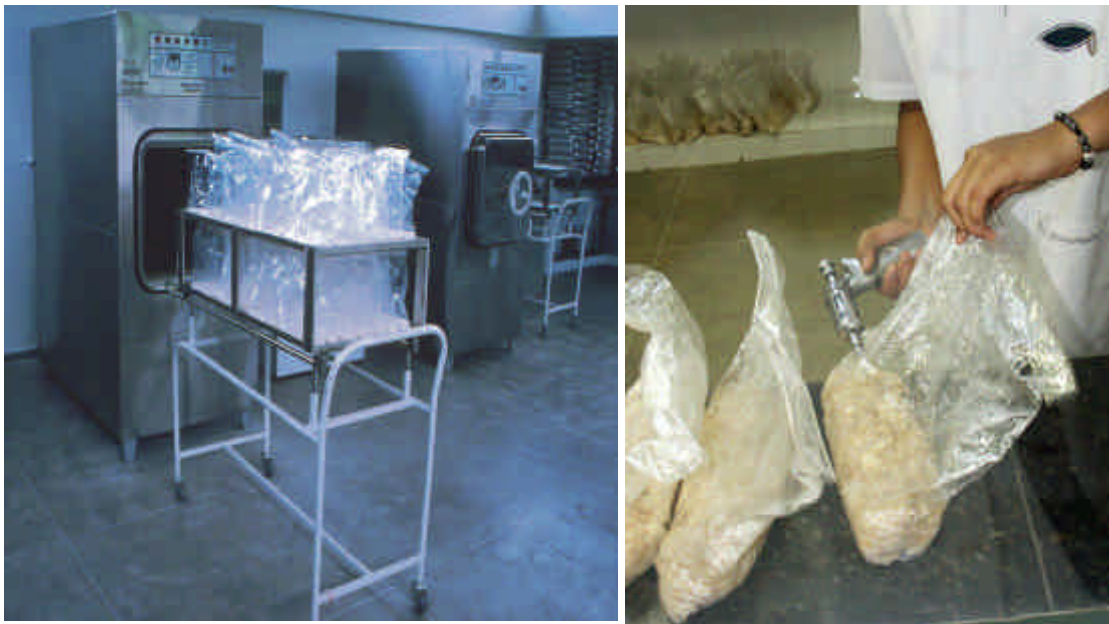
Fig. 2. Autoclave (left) and semi-automatic substrate bag inoculation at CEPLAC, Brazil.
