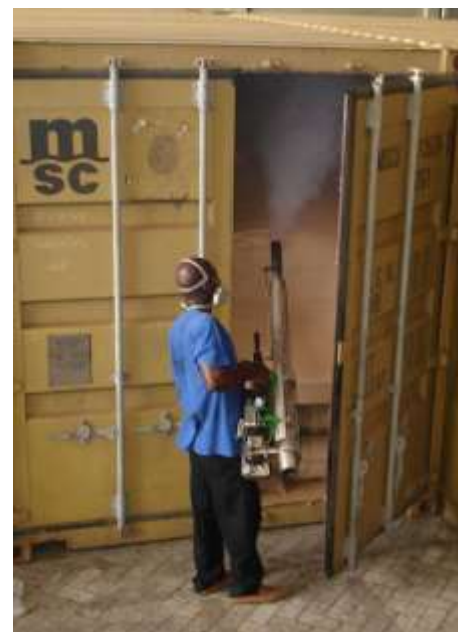
b. Space treatment with a pyrethroid UL formulation: using a thermal fogger before closing the container
