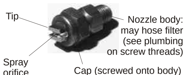
Fig. 1. Housing the nozzle tip
